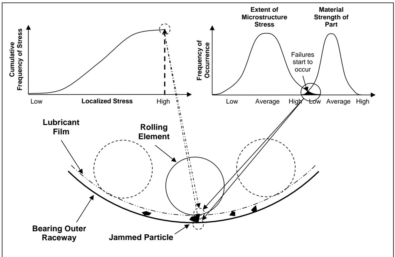
Figure 3.7—Solid Contaminant between Roller and Raceway Overloads the Microstructure]
