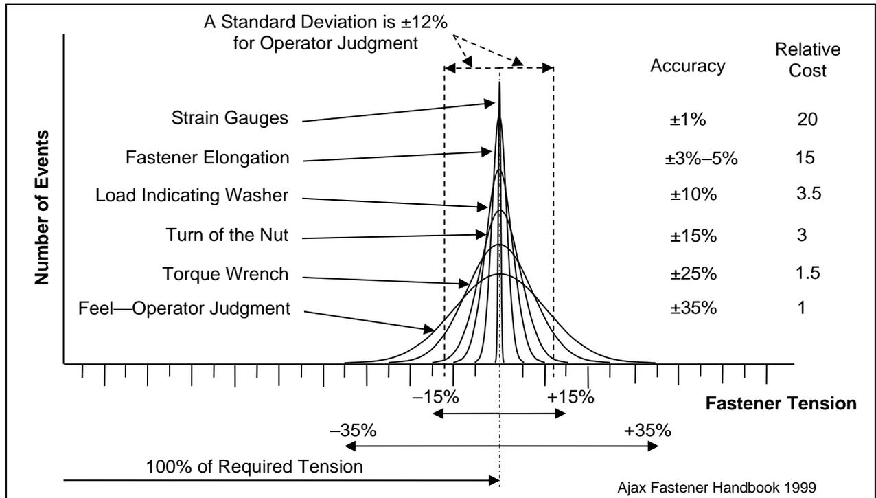
Figure 3.6—Variability in Methods of Providing Correct Torque for Fasteners
