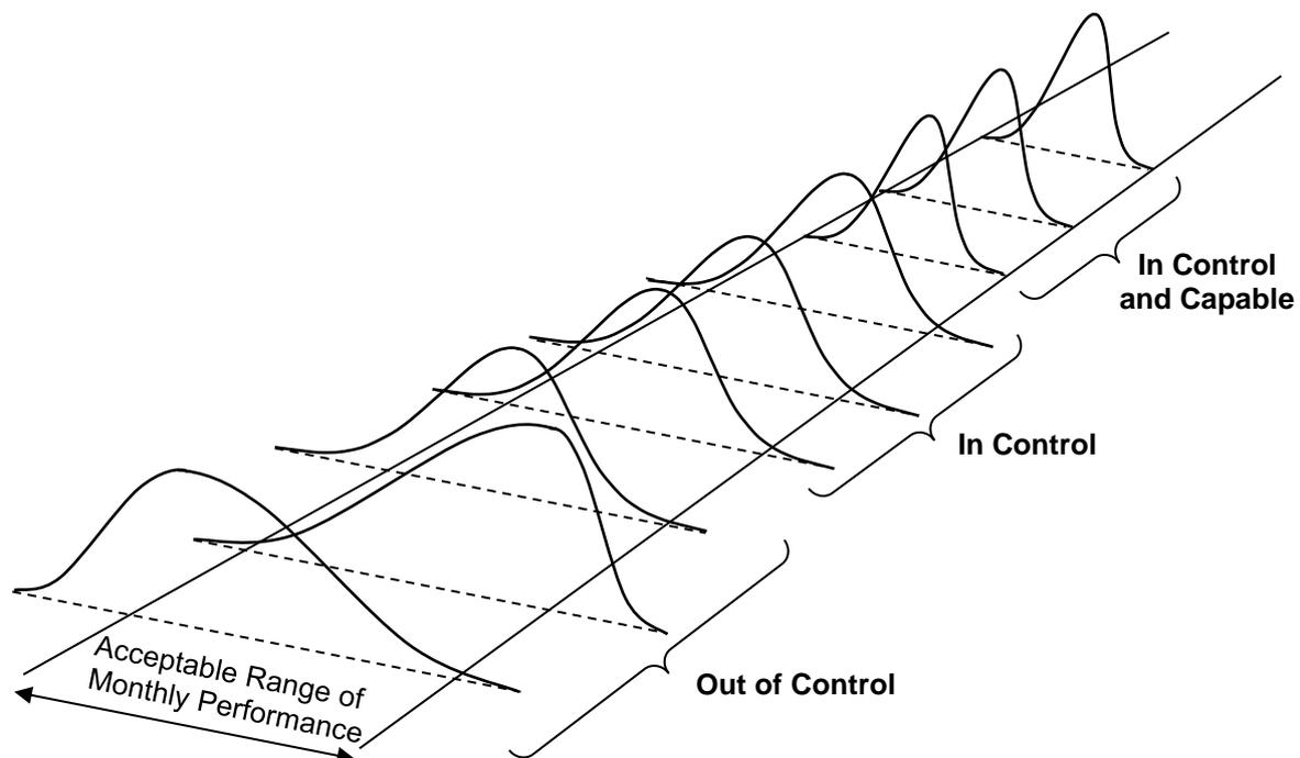
Figure 3.14—Making a Process in Control and Capable
