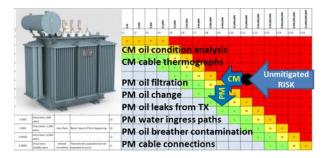
The transformer in the slide gets protection only if the maintenance done is useful for reducing the risk of its failure. Starting at the unmitigated risk point you plot and trace the financial benefits that each work order brings the company. Condition Monitoring (CM) work is a consequence reduction strategy. Proactive Maintenance (PM) work is a chance reduction strategy. The financial benefit of each scheduled maintenance work order must be identifiable on a risk matrix.
