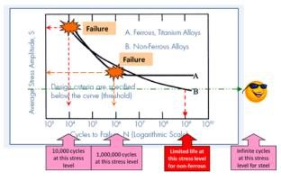
Material fatigue curves tell us what to do to get a long service life for our machine parts. The curves in the fatigue diagram above show that 40% reduction in stress delivers 100 times more service life. They prove that if you lower the atomic stress in materials you will create massive reliability growth.
